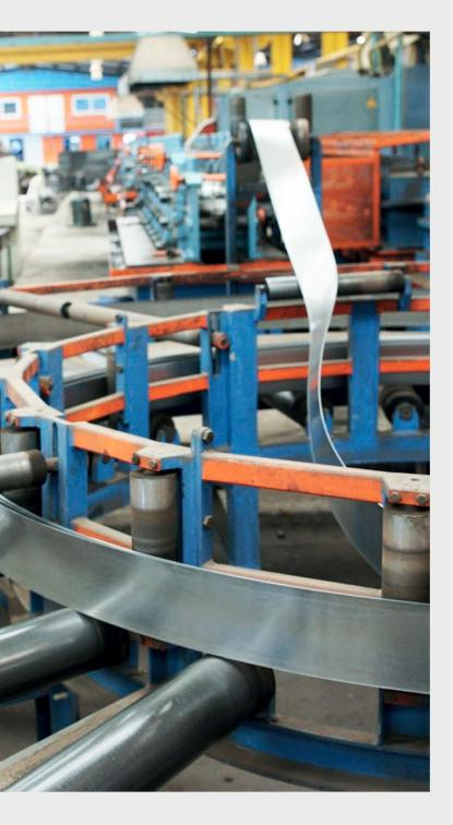
Our pipe factory use Electric resistance welded (ERW) process by cold-forming a sheet of steel into a cylindrical shape to manufacture the pipes and tubes. This factory has four pipes production lines and one Hydro test line.
